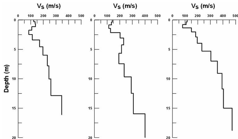
Figure 4. Inverted  $V_s$  from (a) Mardyke GAA pitch, (b) Fitzgeralds park and (c) Mardyke bridge
